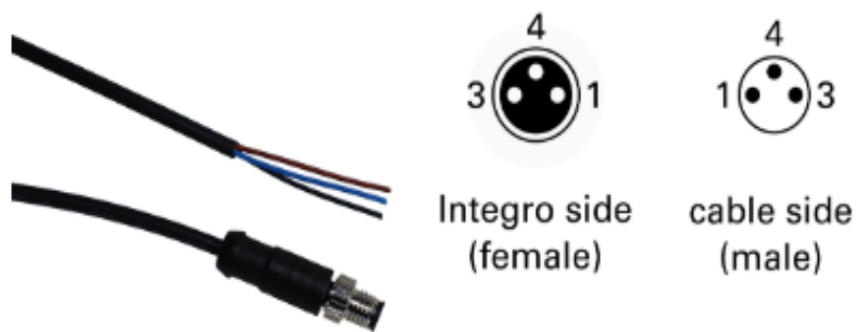
STO/SBC input connector from both SOMANET Integro and cable perspectives (This is an M8 3-pin A-coded connector.)
